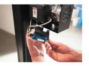
Unscrew and pull out the controller module - remove four screws at the bottom of enclosure (no need to disconnect cables from controller, it can be left out of enclosure by hanging on the cables).
