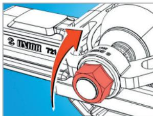
Pričnemo privijati matico zgloba saj s tem razstavimo homokinetičen zglob • Start to screw in the nut of the joint with which you dismount the homokinetic joint.
