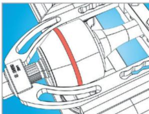
Snamemo vskočnik, ki drži manšeto zgloba • Dismount the circlip which is holding.
