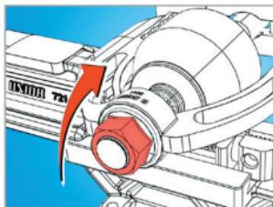
Na navoj zgloba privijemo matico homokinetičnega zgloba • Screw on the nut of the homokinetic joint on the thread of the joint.
