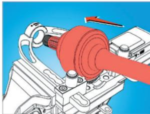
Skozi obroč vstavimo homokinetičen zglob z navojem naprej. Vpnemo lahko zglove z premorom vratu od Ø18 do premera Ø36 • Insert the homokinetic joint through the ring with the threading head ahead. Tool can grasp homokinetic joints with neck diameters from Ø18mm trough diameters of Ø36mm.
